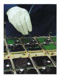
During one of the final stages of production, Essex performs an encapsulation process on each Keypad. This process seals the Keypad circuit assembly, protecting the integrity of the circuit against the elements in even the most demanding environments.
