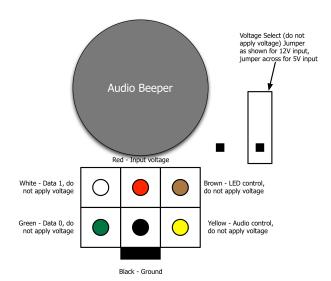
Wiring: Red +5 or 12V DC, see jumper setting
