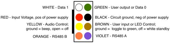
**CAUTION:** Do NOT run this low voltage wiring in conduit with or adjacent to line voltage wiring.
